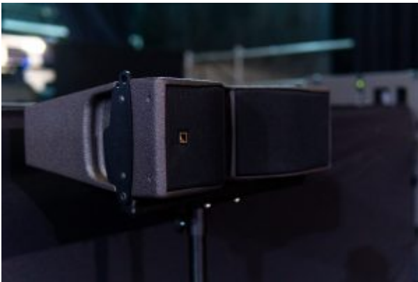
Close up of the L-Acoustics Kiva II front-fill.
