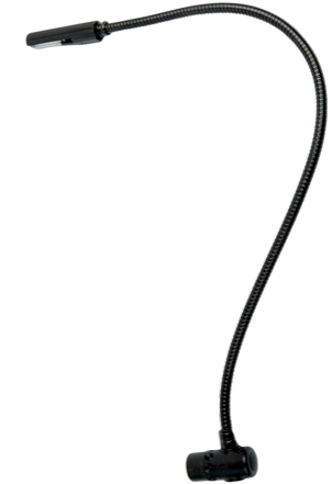
18XR-4-LED CONSOLE LIGHT Littlite XR-4 Series console lights configured for the MIDAS PRO2 series audio consoles. 18XR-4-LED ML for left side of PRO2. Important Note!: The Littlite PRO2 series lights are configured for the first generation PRO2 consoles. Later generations may have different XLR panel socket orientations and require the pin inserts in your Littlites to be rotated to match.
